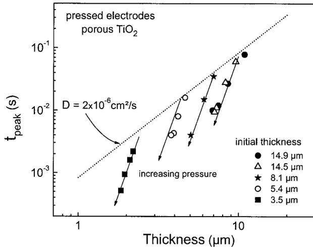
FIG. 7. Dependence of  $t_{\text{peak}}$  on the layer thickness for pressed electrodes with different initial thicknesses. The pressures were 0.2, 0.4, 0.6, and 0.8 t/cm<sup>2</sup>. The dotted line gives the dependence for  $D=2 \times 10^{-6}$  cm<sup>2</sup>/s.
