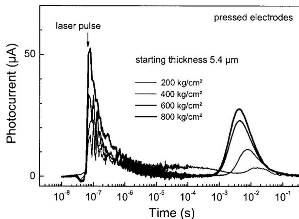
FIG. 6. Photocurrent transients of pressed porous TiO<sub>2</sub> electrodes with initial layer thickness of  $5.4 \mu\text{m}$ .
